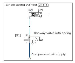
Fig 4: Pneumatic circuit using single-acting cylinder (Cl 1-1). Simulation
