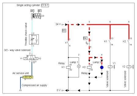
Fig 10: Electro-pneumatic circuit with cylinder (Cl 3-1). Simulation II
