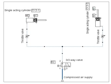
Fig 7: Pneumatic circuit with two cylinders. Simulation
