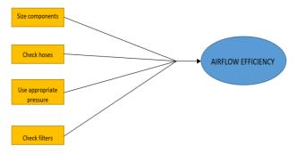
Fig 11: Components of air flow efficiency
