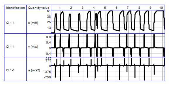
Fig 5: The state diagrams of single acting cylinder
