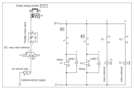
Fig 8: Electro-pneumatic circuit with cylinder (Cl 3-1)
