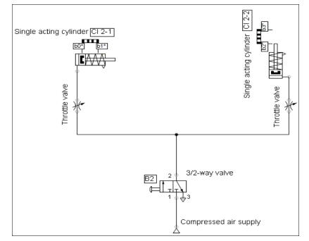
Fig 6: The second pneumatic circuit with two cylinders
