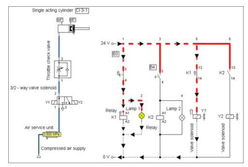
Fig 9: Electro-pneumatic circuit with cylinder (Cl 3-1). Simulation I
