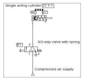
Fig 3: First pneumatic circuit with cylinder (Cl 1-1)
