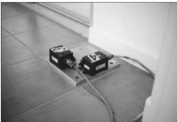
Fig 2: Picture of several accelerometers placed on the ground
