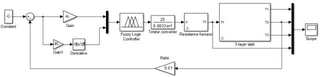
Fig 4: Simulik diagram of slab temperature control system using fuzzy controller PD
