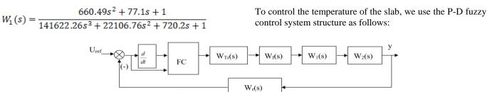
Fig 2: Structure of slab temperature control system
