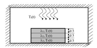
Fig 1: Heat transfer model of furnace
