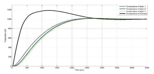
Fig 5: Simulation results of the temperature control system 3-layer slab
