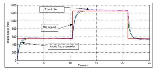
Fig 4: The response between the PID controller and the hybrid fuzzy controller when changing the setting speed
