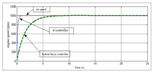
Fig 2: The response between the PID controller and the hybrid fuzzy controller with step function input
