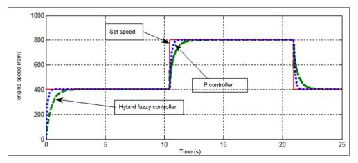
Fig 3: The response between the PID controller and the hybrid fuzzy controller with square function input
