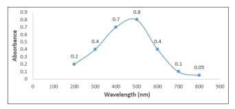
Fig 1: UV-visible spectrum of Ag/Ni bimetallic nanoparticles
