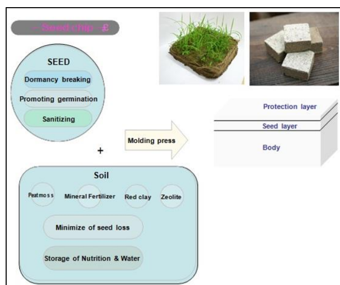
Fig 1: Seed chip structure (was made by research from Kyungpook University-Korea) [7]
