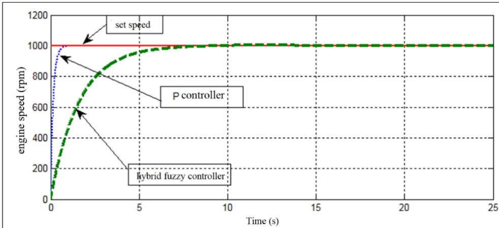
**Fig 2:** The response between the PID controller and the hybrid fuzzy controller with step function input
