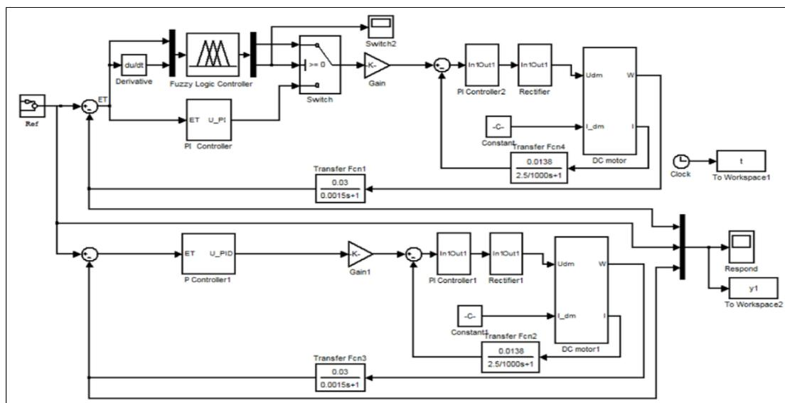
Fig 1: Structure simulation of the response between the PID controller and the hybrid fuzzy controller
