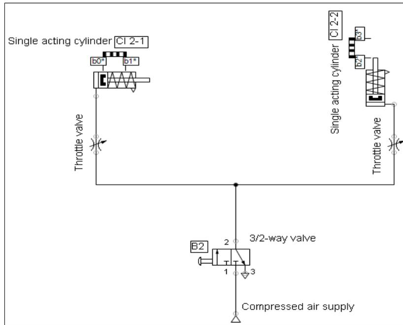
Fig 6: The second pneumatic circuit with two cylinders
