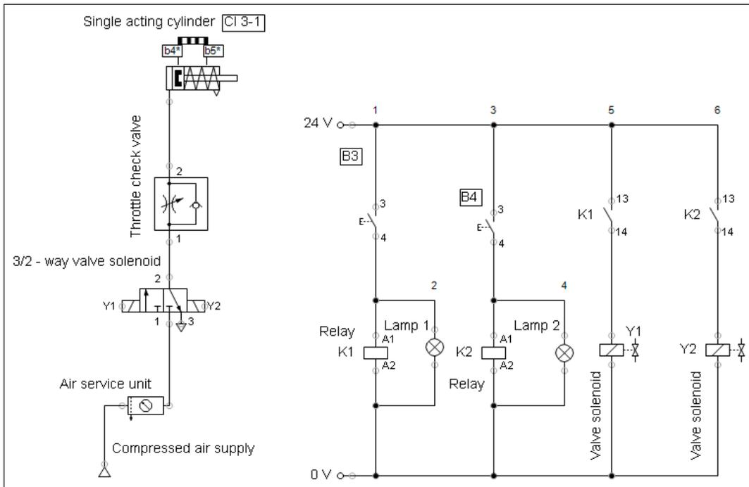
**Fig 8:** Electro-pneumatic circuit with cylinder (CI 3-1)
