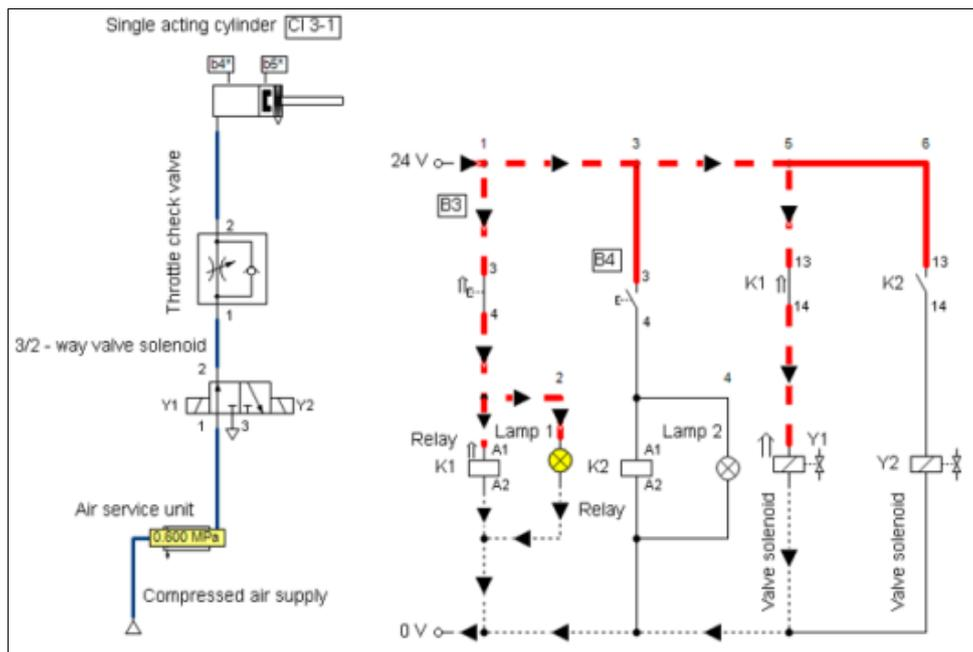
**Fig 9:** Electro-pneumatic circuit with cylinder (CI 3-1). Simulation I
