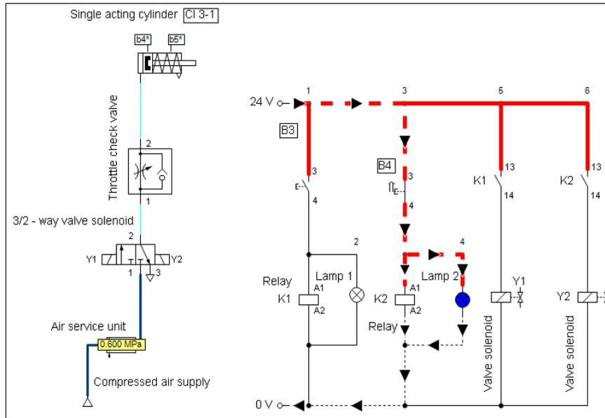
Fig 10: Electro-pneumatic circuit with cylinder (CI 3-1). Simulation II
