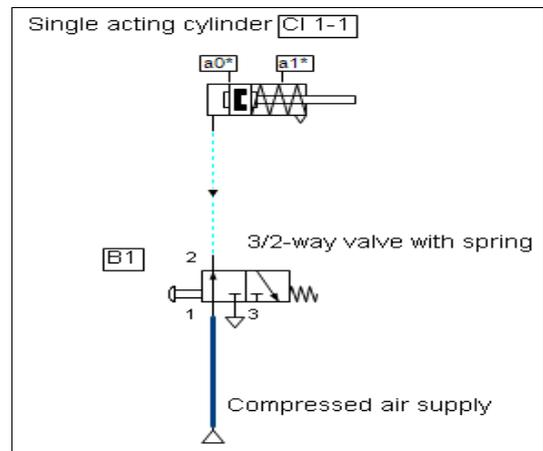
Fig 4: Pneumatic circuit using single-acting cylinder (CI 1-1). Simulation
