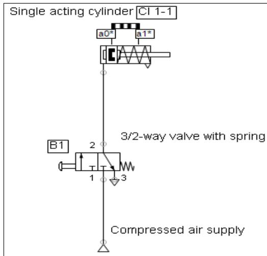
Fig 3: First pneumatic circuit with cylinder (CI 1-1)
