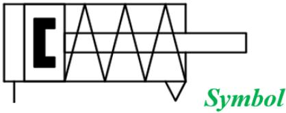
Fig 2: Symbol of single-acting cylinder
