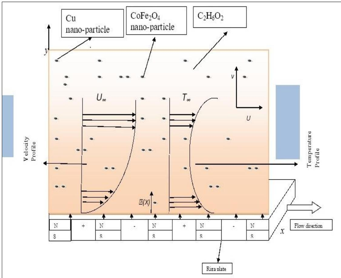
Fig 1: Flow model of hybrid nanofluid in a stretching porous medium with Riga plate
